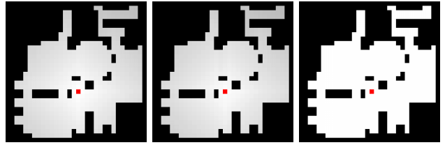
Fig. 8. On the left ground truth generated by Value Iteration algorithm. In the middle UNet generated map. Gradients of these maps indicate state values that lead to a positive terminal state. On the right, UNet generated success map. White cells in the success map indicate that there exists a path to a positive terminal state.
