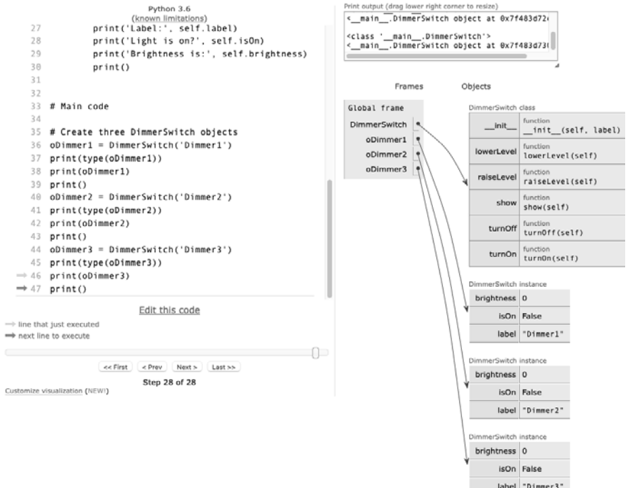
Figure 3-3: Running Listing 3-2 demonstrates that objects do not include code, in accordance with mental model #2.
