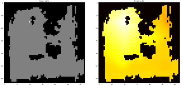
Fig. 12. Discretized map from LIDAR point cloud on 2D plane on the left. The map of values of states after passing through UNet-RNN-Skip model on the right.
